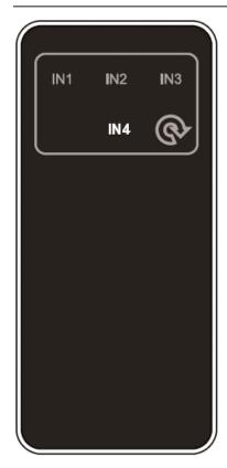
IN1/2/3/4: Press IN1/2/3/4 button to select HDMI signal source INPUT 1/2/3/4 to the OUTPUT port.
