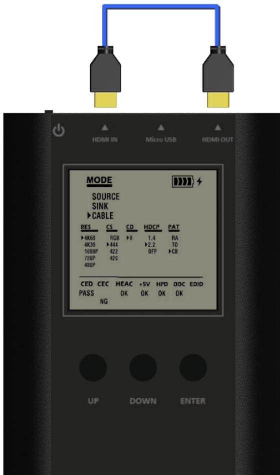
In this mode, BG-AVTPG-MINI offers a link quality estimator using a Character Error Detection mechanism to HDMI 2.0 specifications. The estimator can provide a basic link quality evaluation regarding the cable or any other HDMI link connected to BG-AVTPG-MINI.
