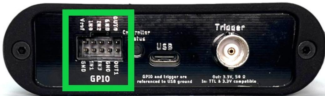
The JS220 software can record the input signals and control the output signals. The input signals allow the JS220 to monitor other equipment and your device under test. The output signals can be used to control other equipment or the device under test. The user interface can display inputs time-synchronized with current, voltage, and power in the oscilloscope view.
