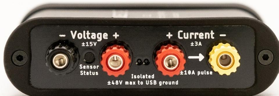
Your JS220 measures the voltage across the Voltage + and Voltage – binding posts. Your JS220 measures the current flowing through the Current + to the Current – binding posts. If you have a power source and target device, connect the positive side through the current binding posts. You can then connect the voltage signals across either your power source or your target device. For more connection examples, see Section 9.
