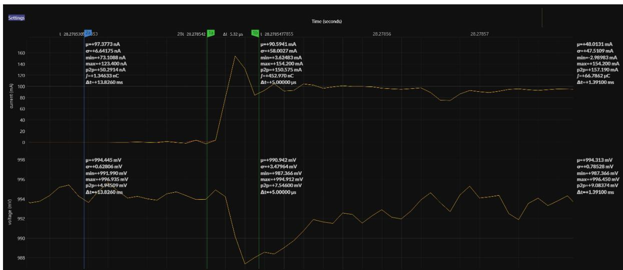
This test shows the current consumption going from 97 nA to 100 mA. The JS220 responds immediately to the change in current. The very slight ripple before the edge is caused by the low-pass FIR filter on the JS220.
