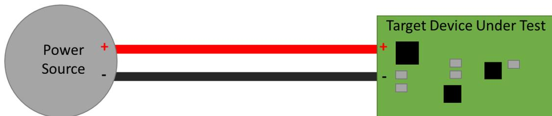
The power source can be anything that provides electricity including a battery, battery pack, rechargeable battery, bench power supply, mains wall adapter, USB, and power regulators.
