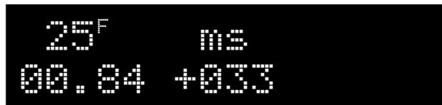
The running average of the current measurement session can also be displayed in milliseconds or frames. This average is calculated on the current measuring session and is not stored.
