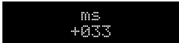
If a frame rate has been set, the reading is also given in frames. Using the same example, with a frame rate of 25 frames the audio is ahead by 00.84 frames.
