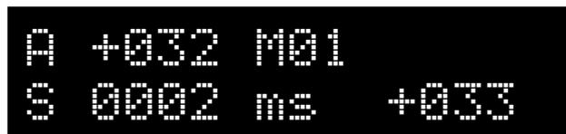
Should the span reading be high, say over 25ms this may suggest there could be inaccurate/anomalous results within the memory buffer. Details of how to go through the memory buffer and remove any suspect readings is given in Show Stats menu item section of the guide on page 11.
