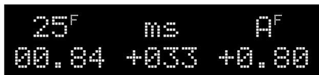
Two flags could also be shown, which indicate when a manual offset and/or speaker distance has been entered, more details on these settings are given in the Advanced Operation section below.
